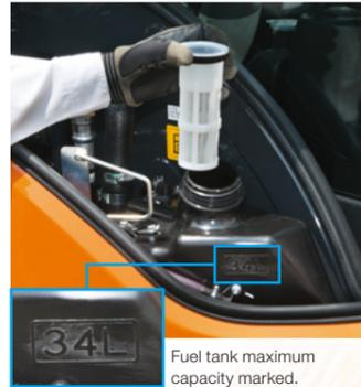
Fuel tank maximum capacity marked.
