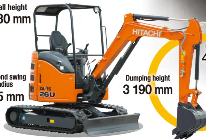
Notes: These specifications are for 4-pillar canopy, 1.17 m arm, extra piping, 0.06 m<sup>3</sup> bucket and 300 mm rubber shoes.
